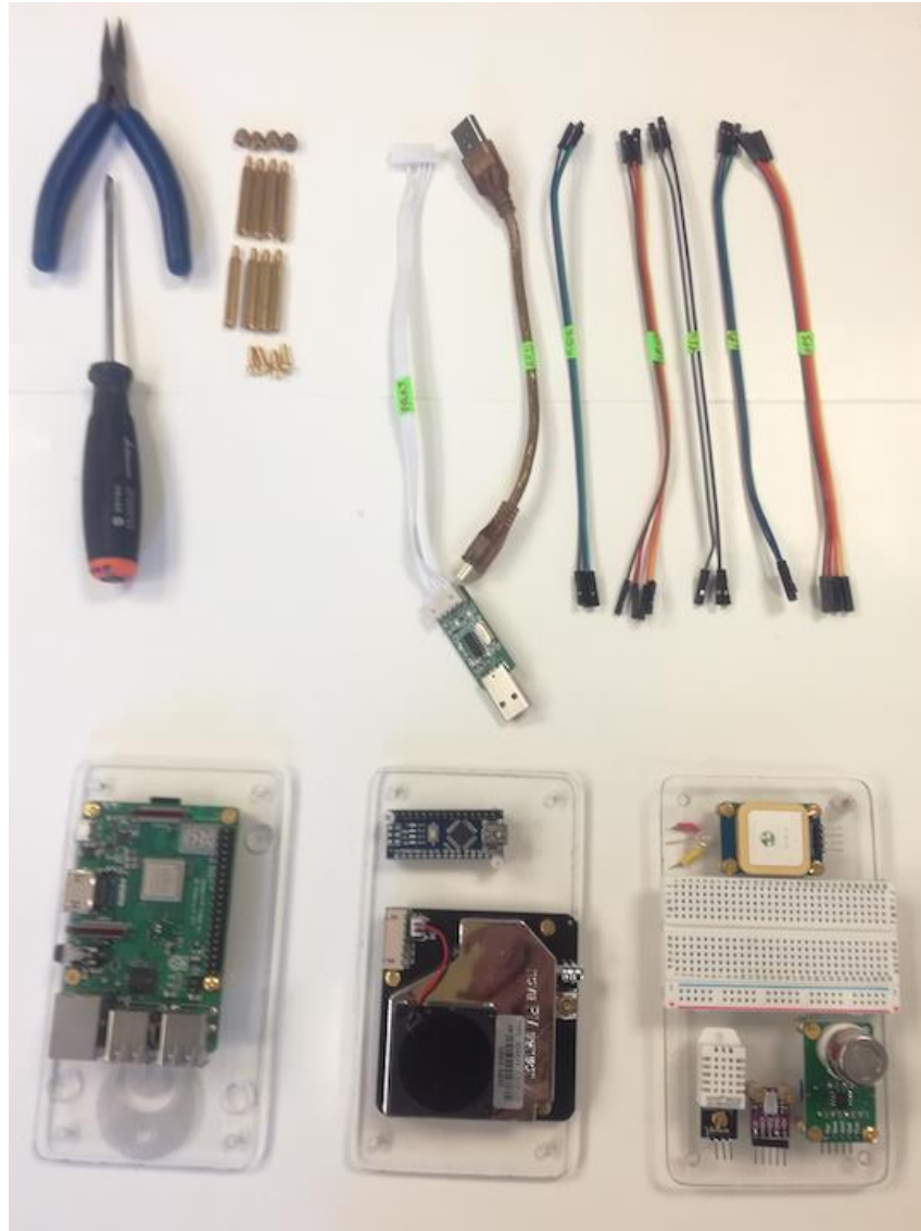
Three layers of AQ Station plus cables, screws and tools (not included in delivery)
