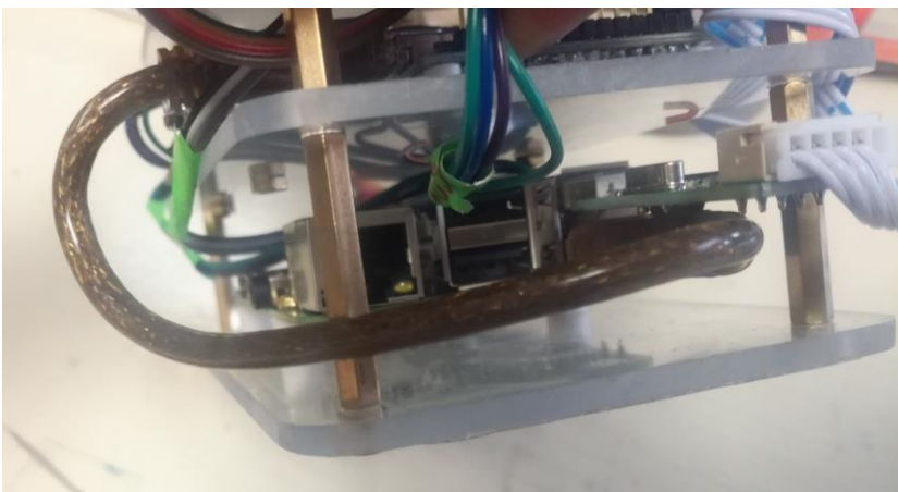
Connecting PM Sensor and microcontroller USB cables to Raspberry Pi.
