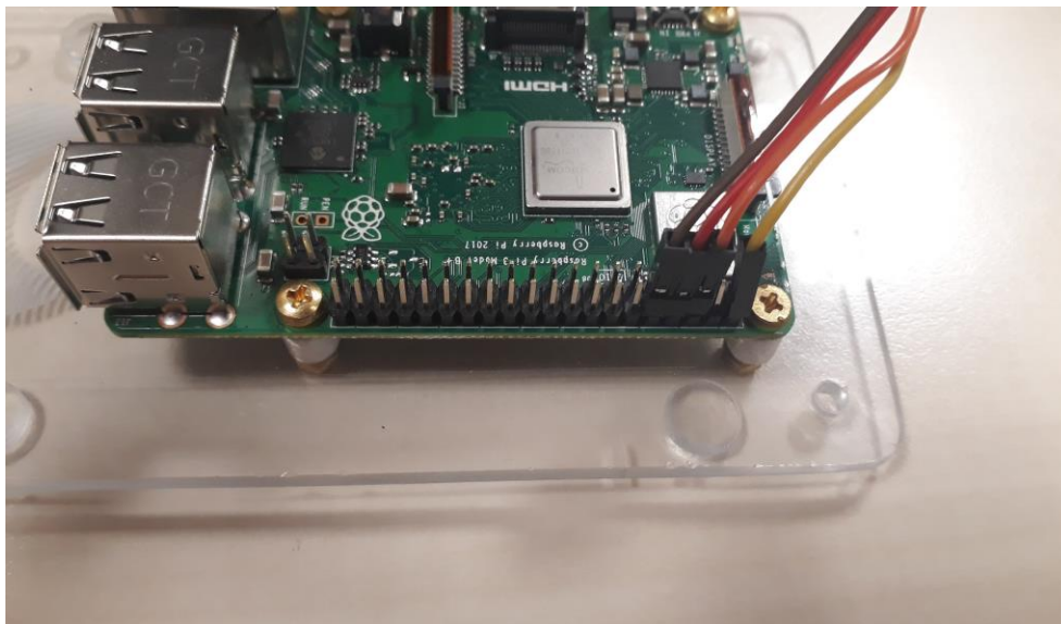
GPS cable connection
